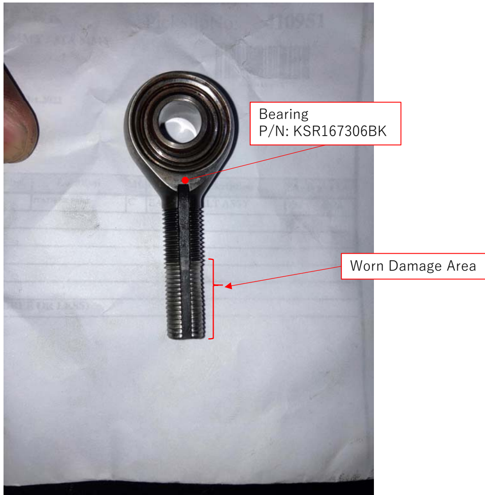
Figure 1 - JA05RK_Worn Damage – Lower Bearing Thread of No.6 Flap Track Fairing Drive Rod
