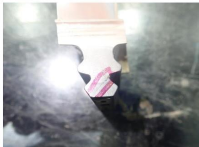
Dovetail area found with crack
