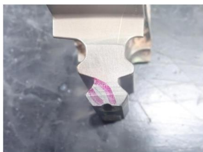
Dovetail area found with crack
