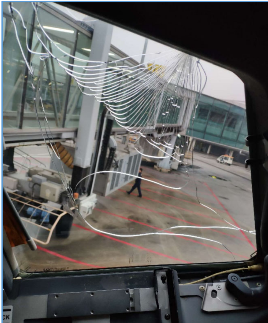
Thermal edge break fracture pattern, typical.
