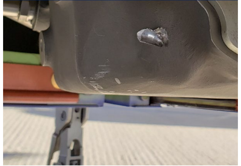
Gouge Damage on TGB (Redesigned Pin)
