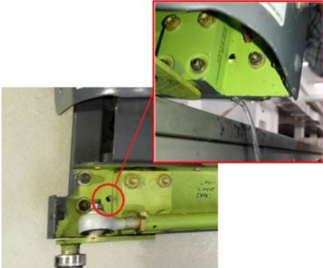
Clean Drain Holes in Window Frame Assembly:
