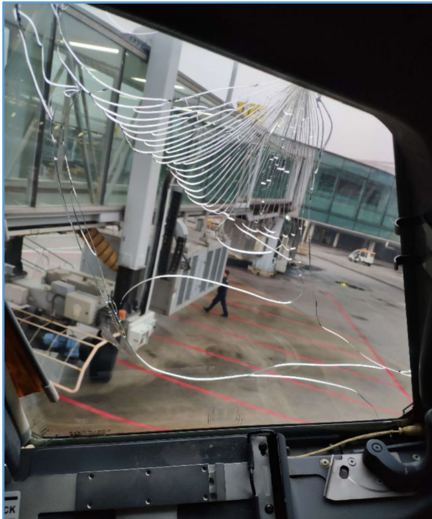
Thermal edge break fracture pattern, typical.
